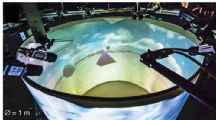
Fig 2. (A) Free flight chamber in which the insect flies toward a skylight cue and with a controlled and measurable downward laminar draft resulting in the subject flying in a horizontal circle within the chamber (Kennedy and Booth 1963, Blackmer and Phelan 1991). (B) Free-flight arena that projects realistic landscapes and monitors insect flight with video-tracking software (Stowers et al. 2017). All images used with permission.
